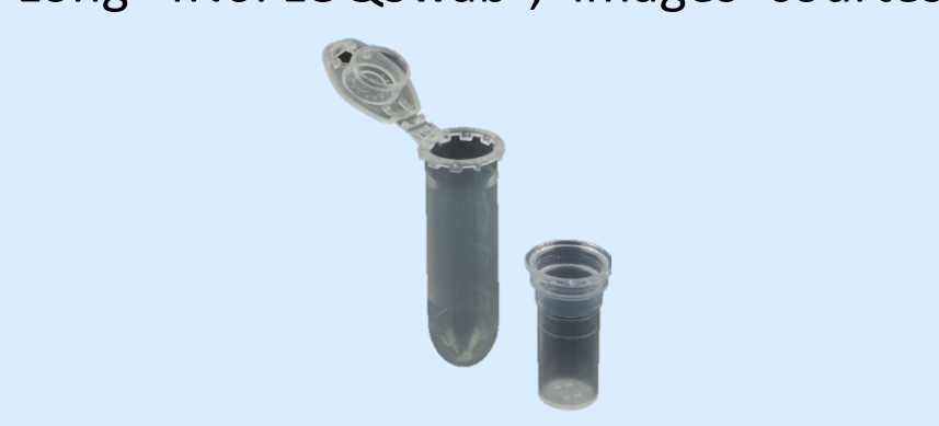
Figure 2: NAO spin basket used during lysis; image courtesy of www.copangroup.com.
